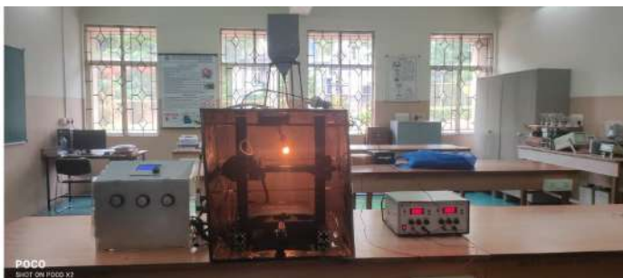
Photograph 6.21: Retrofitting of 3-D Printer for ready to serve baked cakes
