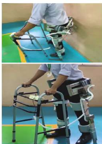
Photograph 6.16: Design and fabrication of Exoskeleton for assistance in walking
