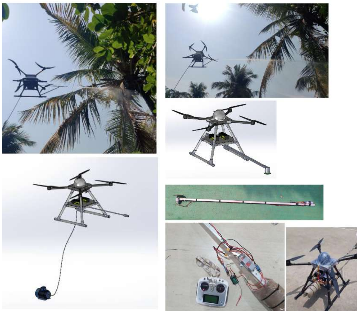
Photograph 6.17: Design and Development of UAV for the harvesting of coconut
