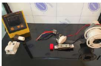
Photograph 6.1: Converting Plastic Waste Bottles to 3D Printing Filament
