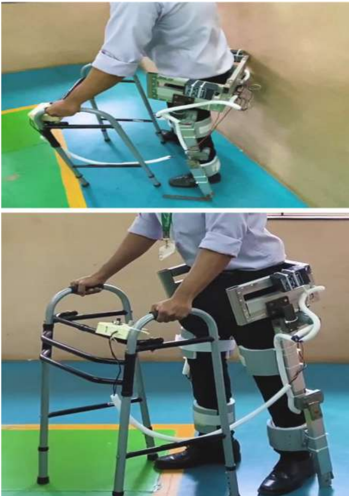
Photograph 5.15: Design and Fabrication of Exoskeleton for Assistance in walking
